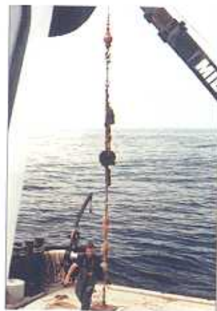
Left: Retrieving an array that holds the receiver. The array is also composed of mooring and a pop-up buoy.
