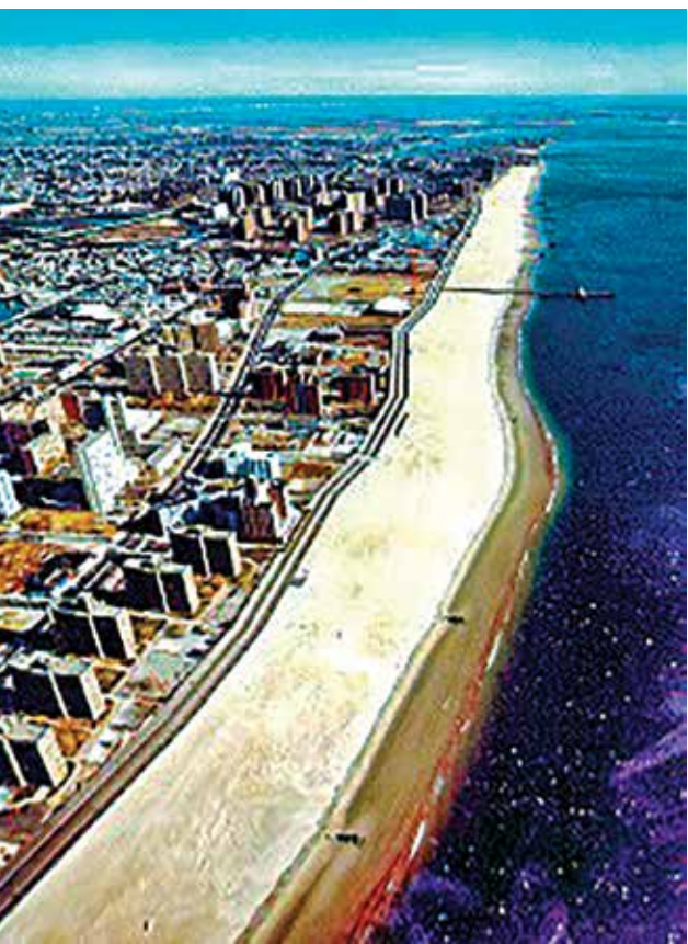
Coney Island Beach after the U.S. Army Corps of Engineers, New York District replenished sand in the early 1990s.
